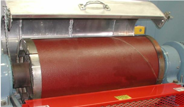
The position of the pressure roll in respect to the cylinder is controlled by micrometer had-wheels graduated in .001". The adjustment is so accurate that print can be sanded from ordinary newspaper without harming the paper itself.
